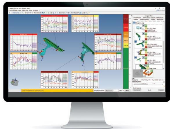
Figure 2: TSAF in eMMA: Classification and filtering of features based on tolerance utilisation
