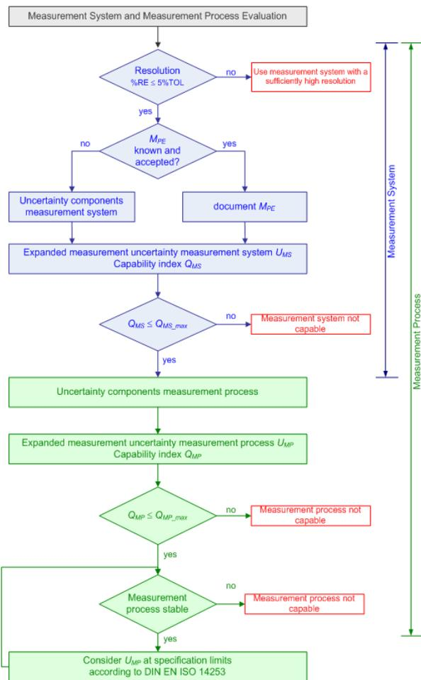
**Figure 6: Approach according to VDA Volume 5**
