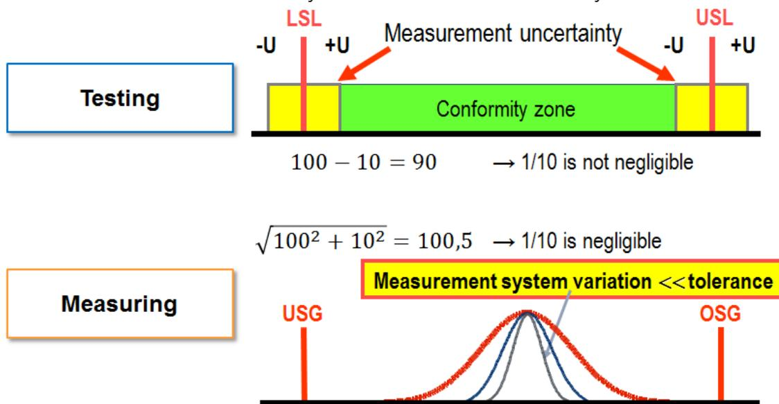
Figure 5: How measurement uncertainty affects a test and a measurement process
